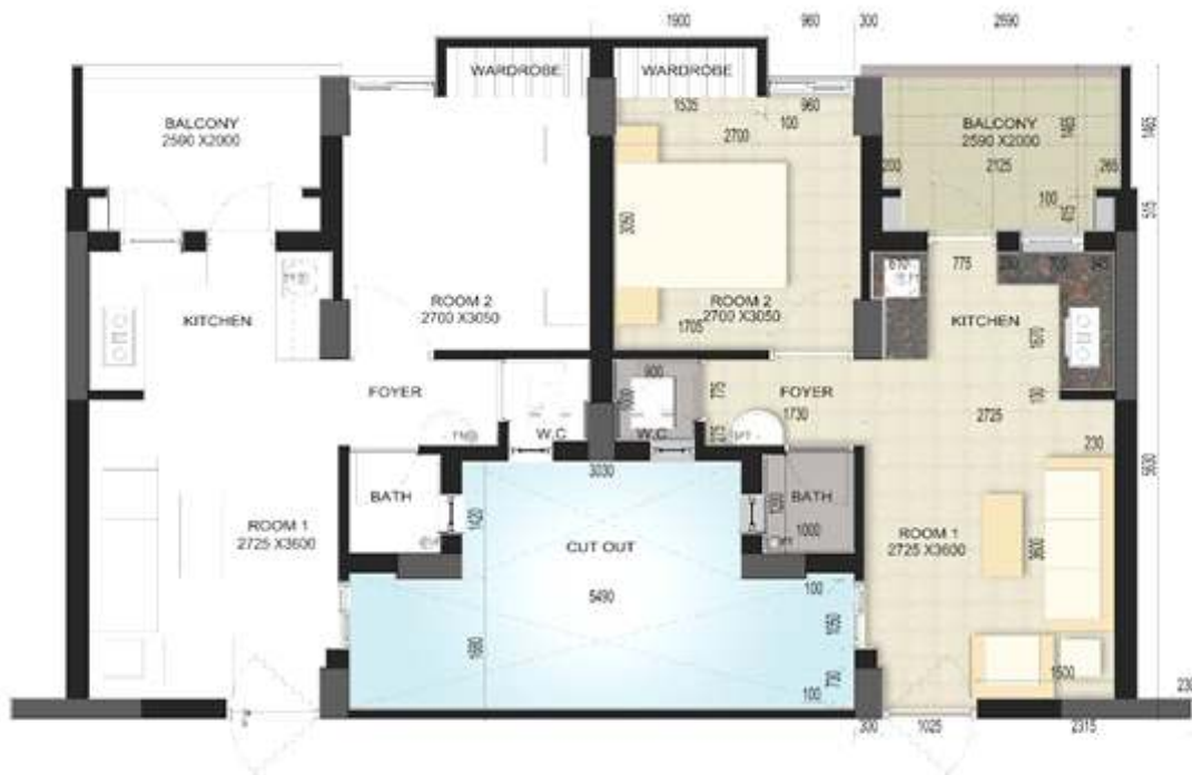
PROJECT: INTEGRATED COMPLEX OF MULTISTOREYED EWS HOUSING WITH FACILITY BUILDING BEHIND DDA PROJECT OFFICE AT MANGLAPURI (SITE NO.IV) TYPICAL UNIT DETAIL
